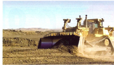
Using specially developed software and GPS guidance systems on dozers, BHP Billiton's La Plata mine restored mined desert lands efficiently and cost-effectively.
