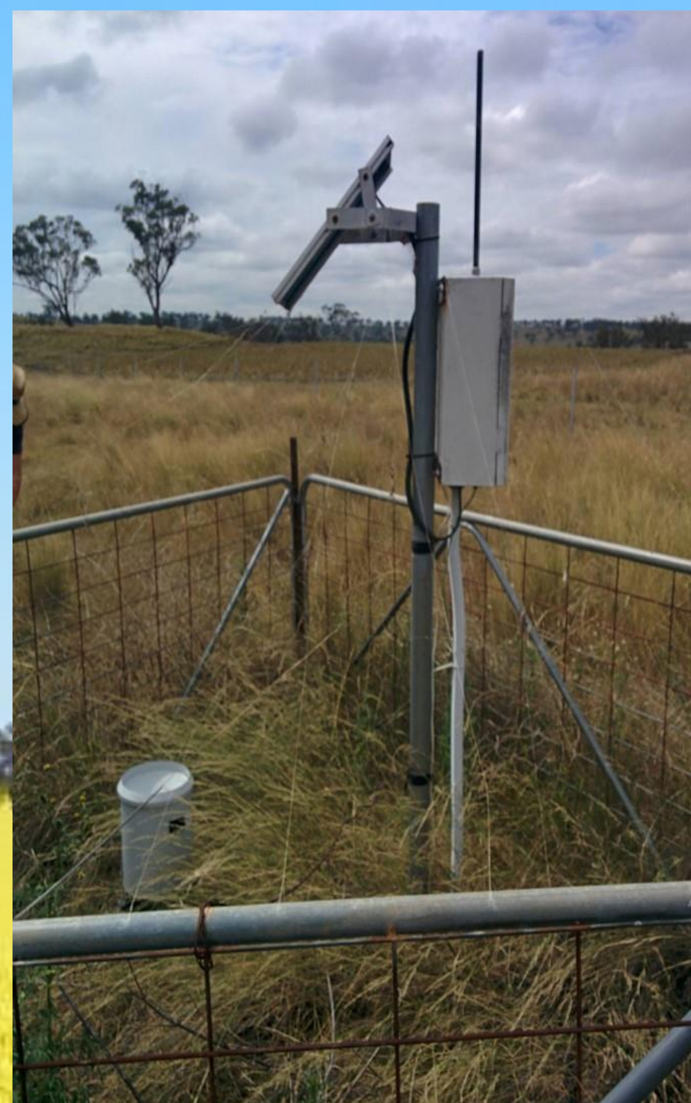
Figure 2. Soil moisture monitoring device on the SAMAS catchment
