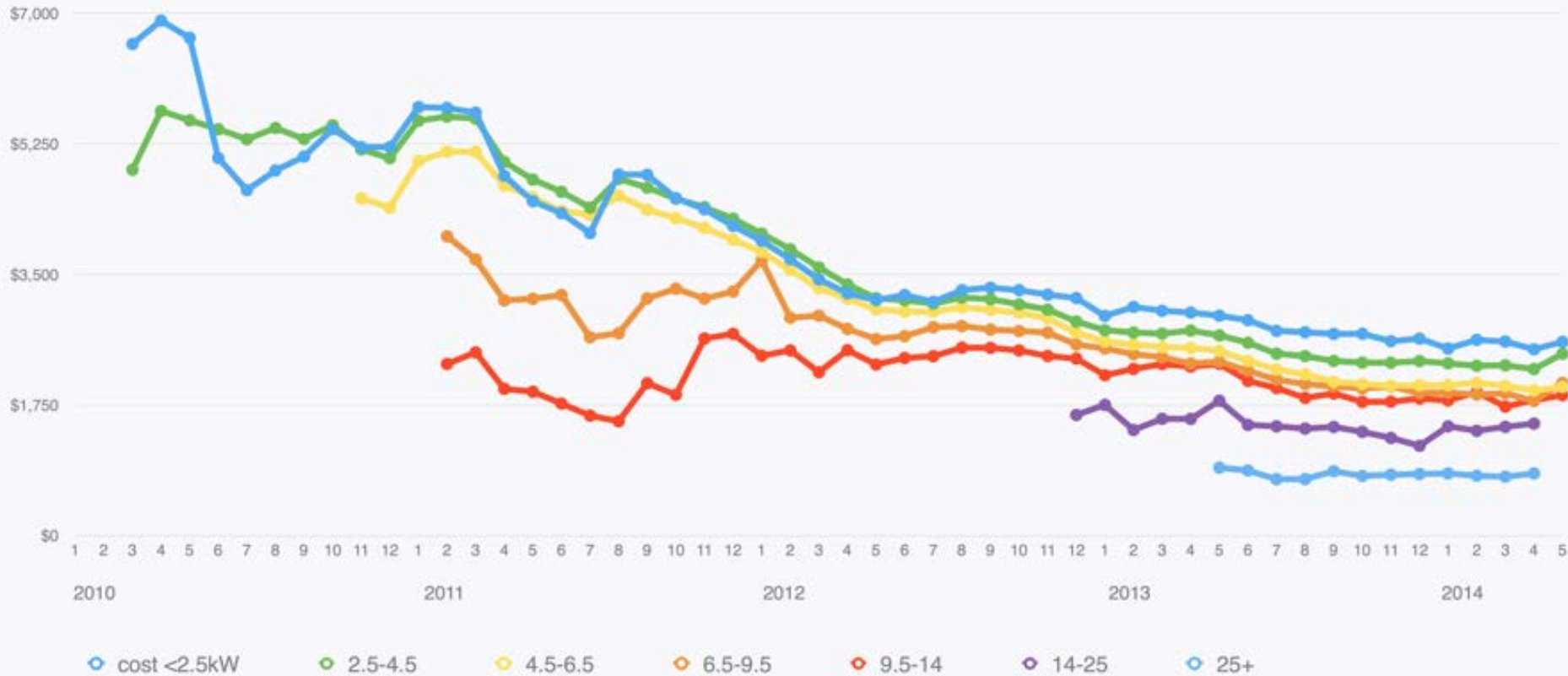
Cost per kW installed, by size category
